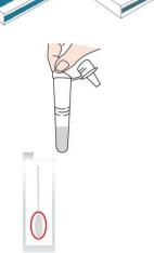
3. Peel off the foil seal from the top of extraction tube, being sure to keep the extraction tube upright.
